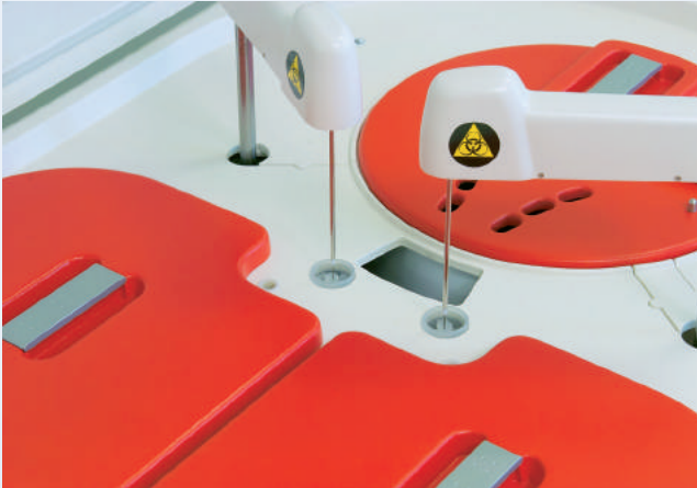
Two independent pipettor arms for a fast and constant workflow
